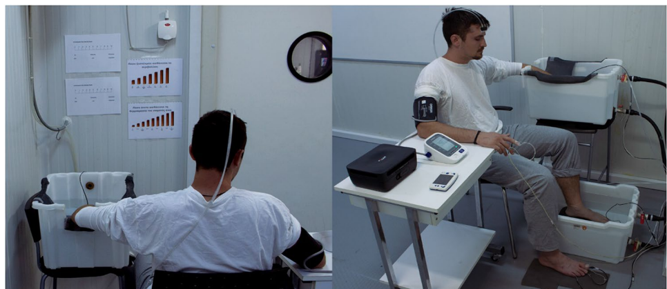
Fig. 2 An able-bodied participant during the data collection. The right sleeve of the shirt was cut at elbow height to avoid constricting blood flow. The blood pressure cuff was comfortably placed at the upper arm without constricting blood flow except when assessing arterial blood pressure
