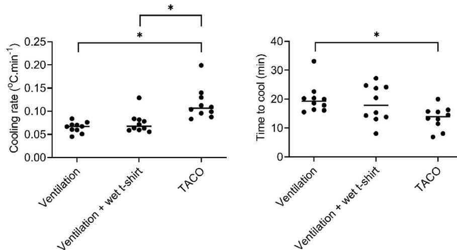
**Fig. 2.** The effect of three different cooling methods (ventilation, ventilation + wet t-shirt and tarp assisted cooling with oscillations; TACO) on cooling rate and time to cool (TTC). Horizontal lines represent group averages. Black dots represent individual data points. \* Denotes a significant ( $P < 0.05$ ) effect of cooling method ( $n = 10$ ).
