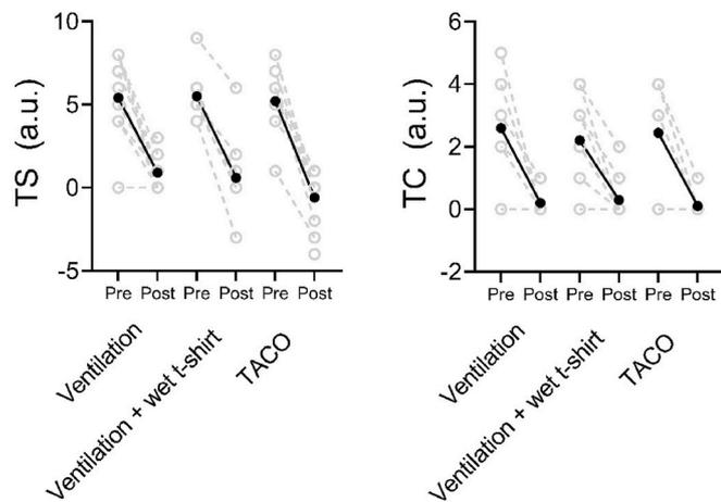
Fig. 3. The effect of three different cooling methods (ventilation, ventilation + wet t-shirt and tarp assisted cooling with oscillations; TACO) on pre- and post-cooling subjective responses: thermal sensation (TS) and thermal comfort (TC). Grey dots and lines represent individual data points. Black dots and lines represent the group average. \* Denotes a significant ( $P < 0.05$ ) interaction effect of time  $\times$  cooling method ( $n = 10$ ).
