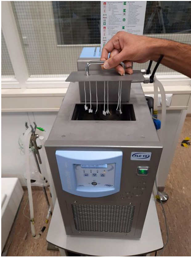
Fig. 2 Setup of the experiment. The sensors were attached to the lid of the Tamson bath
